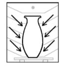
the inside of the ware (and shelves, posts, etc). Conduction is the main way to spread uniform heat through the kiln. It is a slow process.
